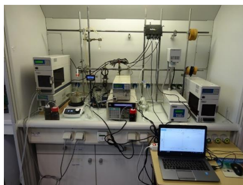
Figure 1. (Left) scheme of the feedback loop for autonomous AI driven optimization. (Right) Prof. Felpin's set-up for autonomous flow optimization.
